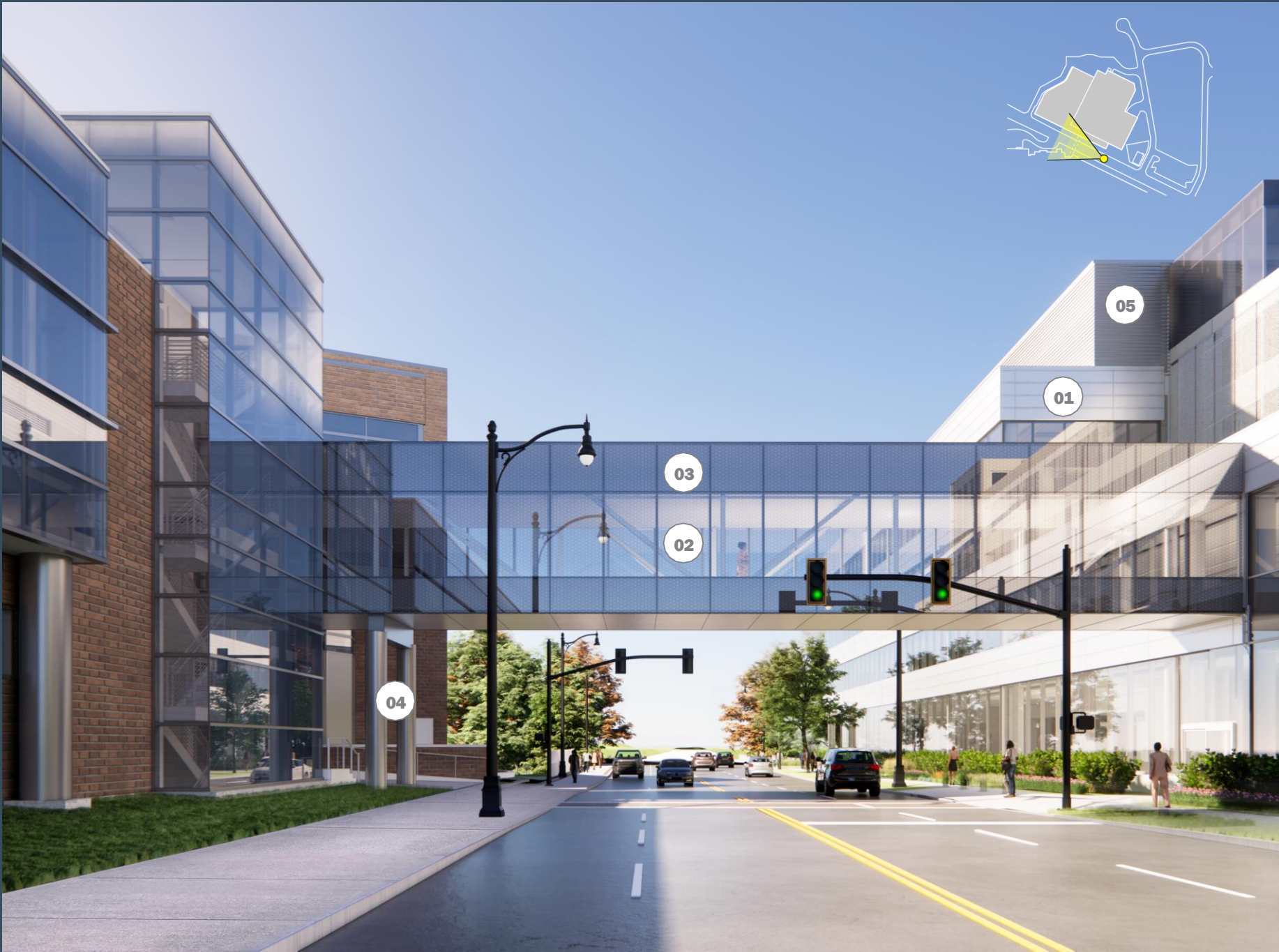
02 CLEAR VISION GLASS - 1/8" DOT S, 2" INLINE BIRD FRIT
